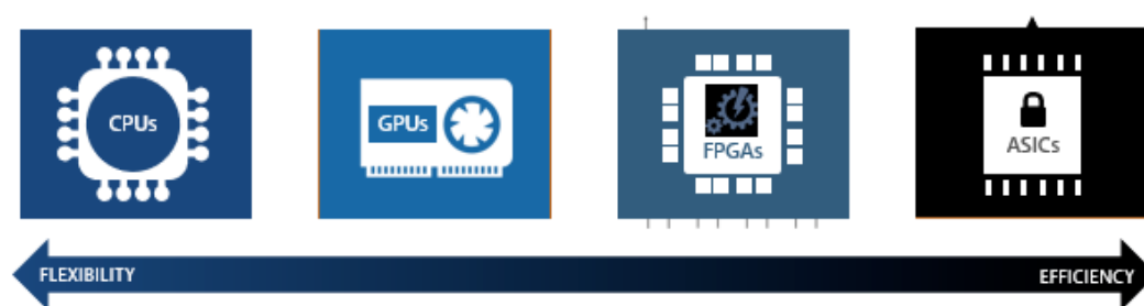
Figure 12: The spectrum of chip architectures with trade-offs in regards to efficiency and flexibility.
